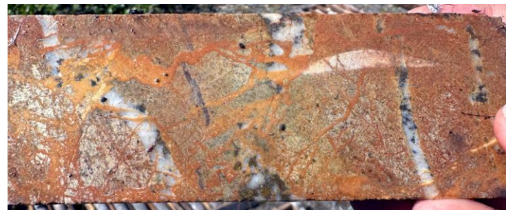
Quartz-sulfide veins cut by carbonate stockwork 0.303 g/t Au 0.19% Cu; 253.1m
