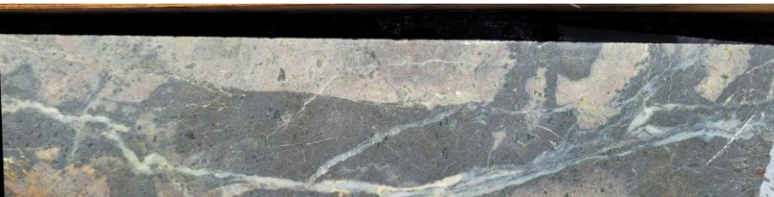
TC20-01 (176 and 219m) quartz calcite and sulfide veins with sericite-pyrite envelopes
