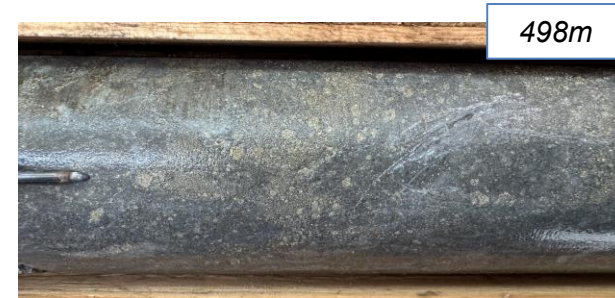
Pyrite flooded feldspar phyrlic andesite: 0.15 g/t Au 2.5 ppm Bi 14.1 ppm Te 23 ppm Se / 3m (495-498m)
