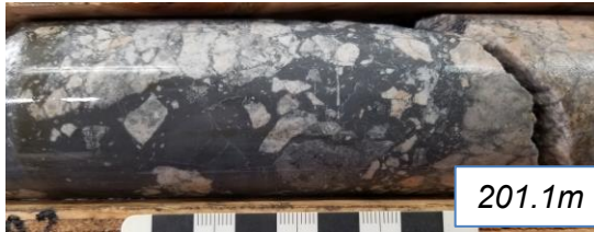
Dacite flow breccia with silicified mudstone matrix
