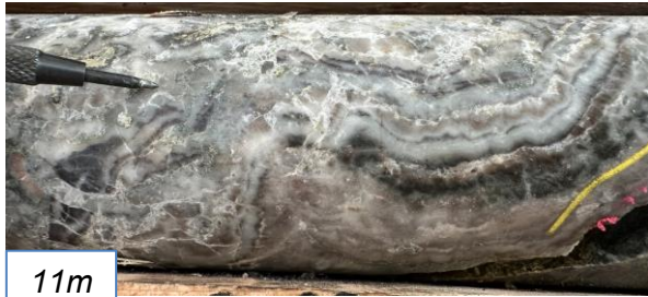
Banded epithermal quartz-carbonate veins: 10.8 g/t Ag 405 ppm Cu 919 ppm Pb 1035 ppm Zn 119 ppm Sb 119 ppm As / 1.m (10-11m)
