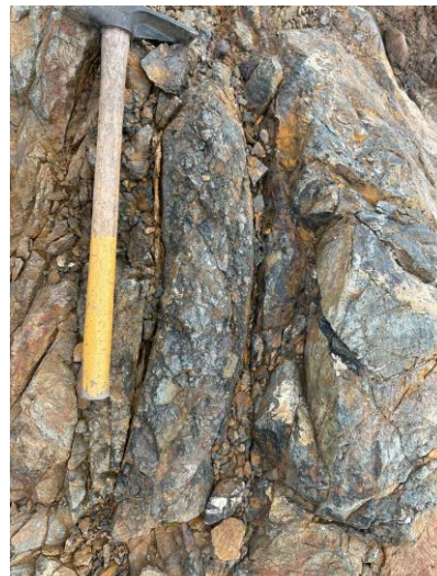
A0420662: brecciated mudstone+sulfides 2.87% Cu
