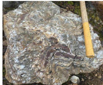
Yellow Bowl Quartz-sulfide vein breccia, 2.92% Cu 25 g/t Ag
