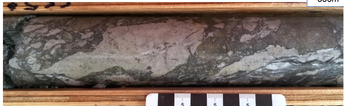
Altered volcanic clasts in sulfide matrix breccia 0.23 g/t Au 498 ppm Cu 2650 ppm As / 3m (531-534m)
