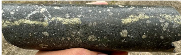
Leucite? feldspar porphyry with coarse chalcopyrite veins 0.07 g/t Au 4480 ppm Cu / 1.36m (191.64-193m)
