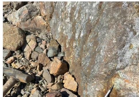
VMS Zone massive sulfide 3.73% Cu, 6.46% Zn, 0.447 g/t Au, 58.2 g/t Ag
