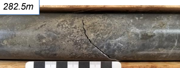
Sericite-pyrite altered dacite 5 ppm Bi 5 ppm Te/ 3m (282-285m)
