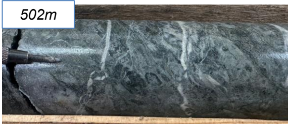
649 ppm Cu 30 ppm Mo 7 ppm Sb / 2m (502-504m)
