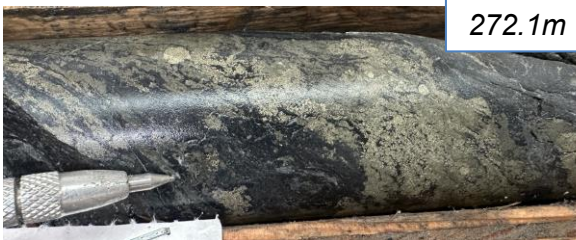
Semi-massive sulfides in mudstone 83 ppb Au 786 ppm Cu 38 ppm Mo 164 ppm As / 3m (270-273m)
