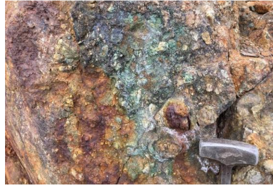
Quartz-sulfide matrix hydrothermal breccias
