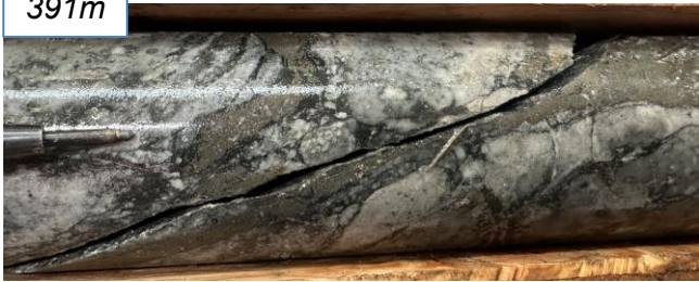
Quartz-chalcopyrite vein in porphyry 86 ppb Au 674 ppm Cu / 3m (373-376m)
