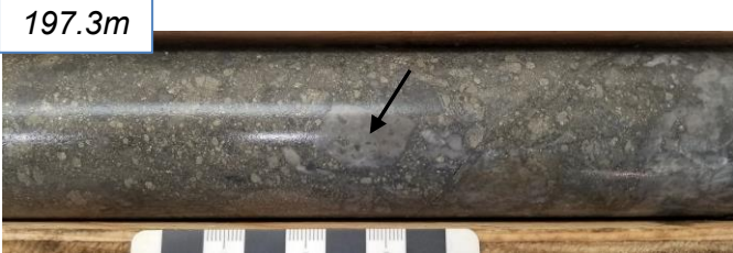
Brecciated semi-massive sulfides with sericite-pyrite altered dacite clasts: 96 ppb Au 29 ppm Mo 343 ppm As 10 ppm Te / 1.68m (197-198.68m)
