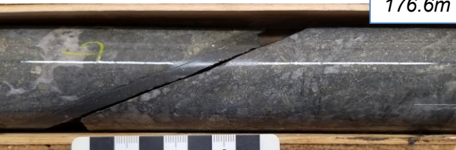
Quartz-calcite-pyrite vein breccia 82 ppb Au 320 ppm As / 3m (174-177m)
