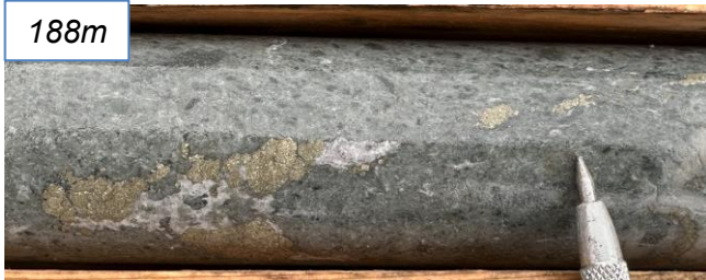
Feldspar porphyry intrusion with pyrite-chalcopyrite blebs
