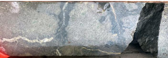
TC20-01 (156m) py-asy and quartz veins in tuff with disseminated py and purple anhydrite
