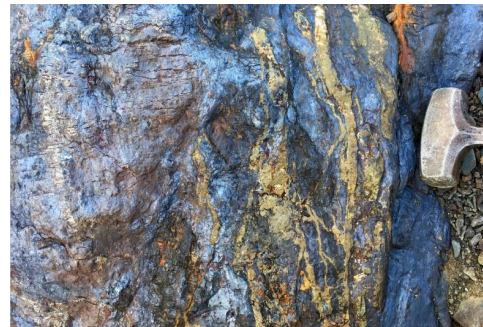
VMS Zone massive sulfide 3.73% Cu, 6.46% Zn, 0.447 g/t Au, 58.2 g/t Ag
