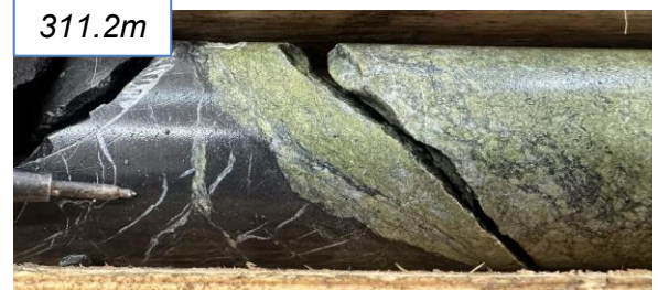
Epidote altered porphyry intruding mudstone 494 ppm Cu 25 ppm Mo 7 ppm Sb / 3m (309-312m)
