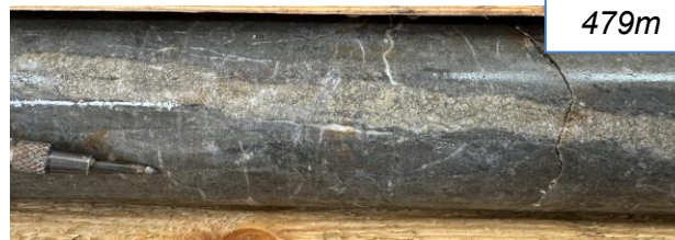
Pyrite-calcite vein in sericite-pyrite-calcite altered volcanics: 18.2 ppm Te / 3m (477-480m)
