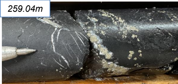
Mudstone with pyrite-chalcopyrite 282 ppm Cu 32 ppm Mo 122 ppm As / 3m (258-261m)
