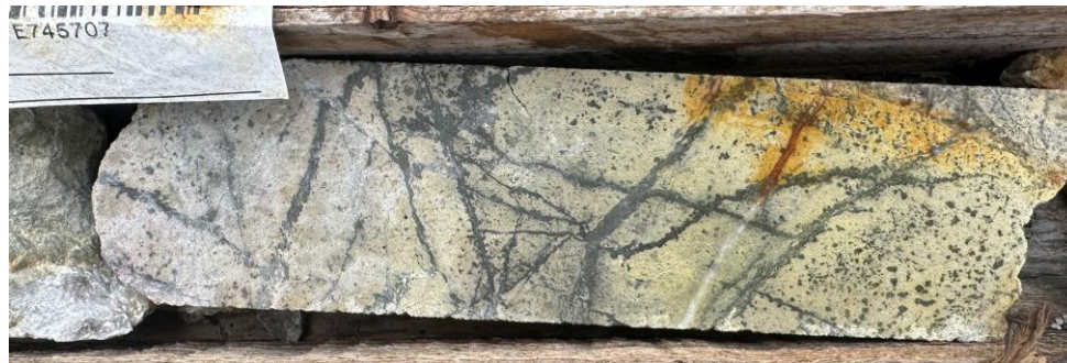
Sulfide stockwork, QSP alteration 0.14% Cu, 0.23% Zn
