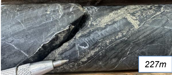
Mudstones with sulfide laminae 3.5 ppm Ag 859 ppm Cu / 2m (228-228m)
