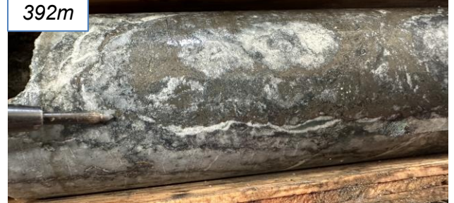
Black chlorite-sulfide veins 358 ppm As 18 ppm Sb / 3m (391-394m)
