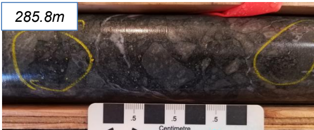
Hyaloclastite with chlorite-sulfide matrix 410 ppm Cu 224 ppm Pb 584 ppm Zn / 3m (283-286m)
