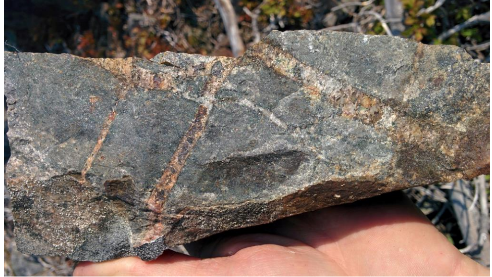
Volcanics cut by multistage magnetite and quartz-sulfide stockwork
