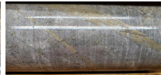
404m Crowded porphyry, py D veins with ser envelopes (pyrite halo)
