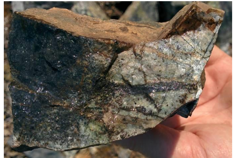
Hornfels with patchy/vein biotite-magnetite-sulfides
