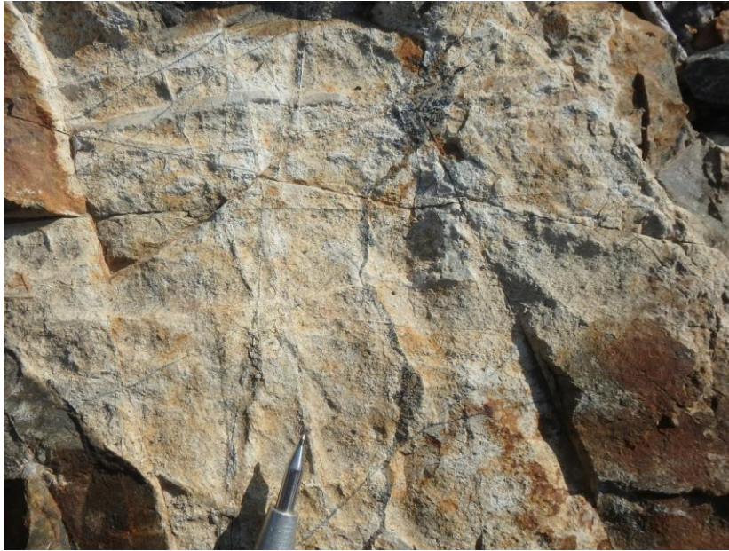
Volcanics cut by multistage magnetite and quartz-sulfide stockwork
