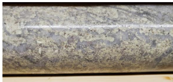
372.5m UST (magmatic-hydrothermal transition texture)
