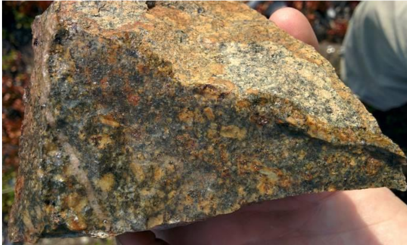
Altered porphyry with quartz-sulfide veins
