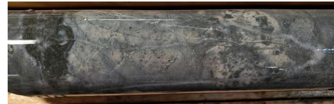
473.3m Fine-grained porphyry/breccia, qtz-mt veins, patchy albite/K-feldspar 0.10% Cu, 73 ppm Mo (0.16% CuEq)
