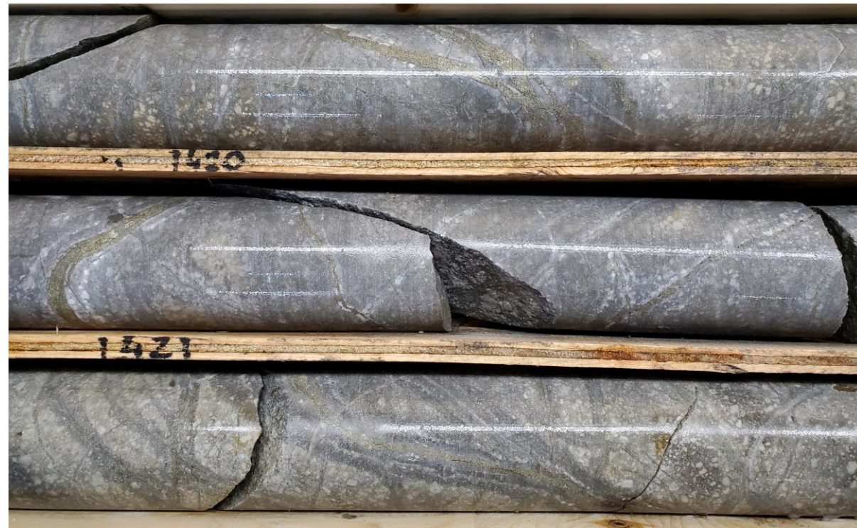
419-421m Crowded porphyry, intense py D veins with sericite envelopes (pyrite halo)
