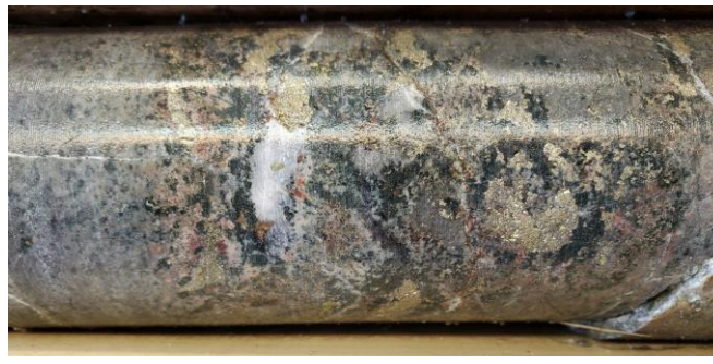
99.7m Breccia, patchy chl-cal-py-cp-mo 0.13% Cu 0.04 g/t Au, 23 ppm Mo, 0.9 g/t Ag (0.18% CuEq)
