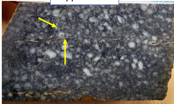
26.9m Crowded porphyry, qtz-cp-mo veins 0.23% Cu 0.19 g/t Au, 95 ppm Mo, 2.7 g/t Ag (0.43% CuEq)
