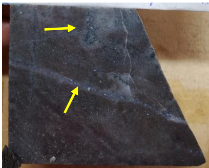
36.3m Crowded porphyry, qtz-cp-mo vein cutting chl(bt)-mt vein 0.13% Cu 0.06 g/t Au, 90 ppm Mo, 1.5 g/t Ag (0.23% CuEq)
