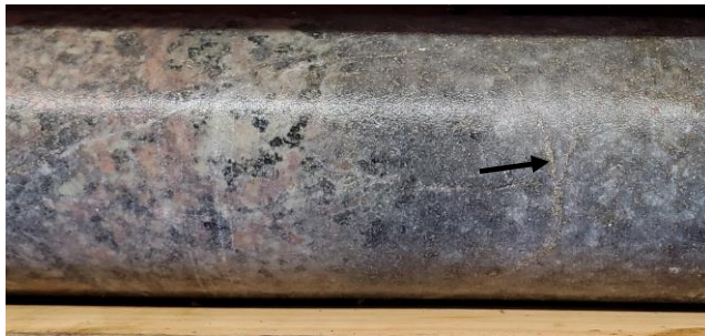
60.3m Crowded porphyry, qtz-py-cp-mo veins 0.10% Cu 0.04 g/t Au, 87 ppm Mo, 0.8 g/t Ag (0.17% CuEq)
