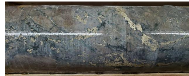
503.4m Strongly hornfelsed andesite, mt-py-cp veins 0.14% Cu 0.04 g/t Au, 76 ppm Mo, 1.0 g/t Ag (0.21% CuEq)
