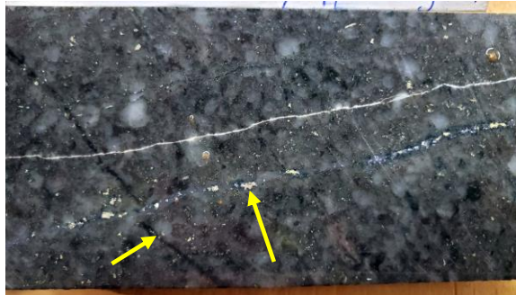
36.3m Crowded porphyry, qtz-cp-mo vein cutting chl(bt)-mt vein 0.13% Cu 0.06 g/t Au, 90 ppm Mo, 1.5 g/t Ag (0.23% CuEq)
