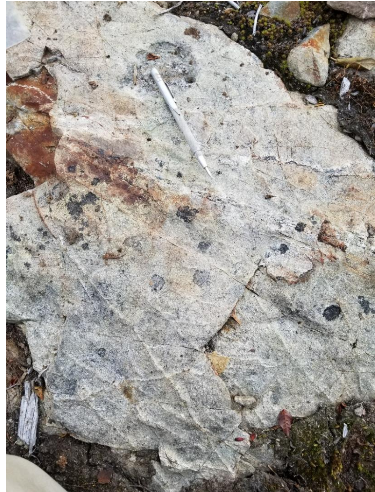
18TRRP003 feldspar-quartz porphyry cut by magnetite-chalcopyrite and quartz-pyrite-chalcopyrite-moly veins
