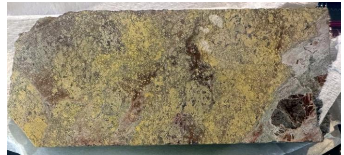
Quartz-sulfide veins cut by carbonate stockwork 0.303 g/t Au, 0.19% Cu; 253.1m
