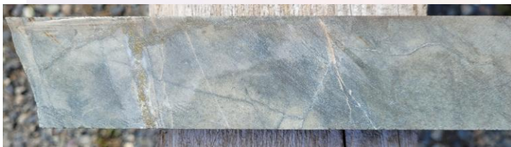
Top TC20-02 (329-338) QSP alteration with dense polyphase veining (up to 0.17% Cu)
