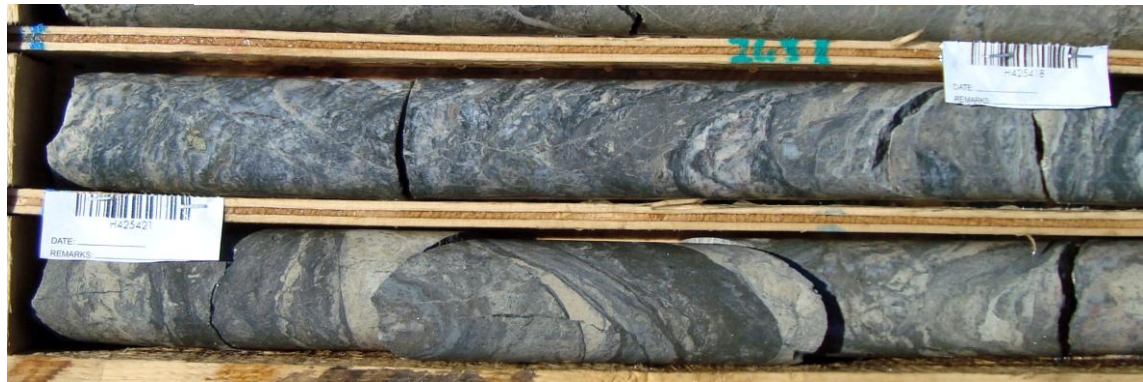
Offcuts and thin section showing potassic alteration at 278m, TC08-03
