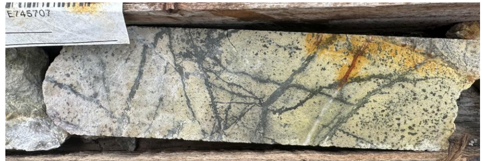
Sulfide stockwork, QSP alteration 0.14% Cu, 0.23% Zn
