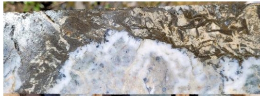
TC20-02 (18.6m) quartz-carbonate-sulfide epithermal vein (0.798% Cu, 23.6 g/t Ag, 0.96% Zn)
