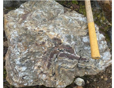
Yellow Bowl: Quartz-sulfide vein breccia, 2.92% Cu, 25 g/t Ag
