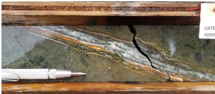
Drill hole photos of NQ core, diameter 47.6 mm
