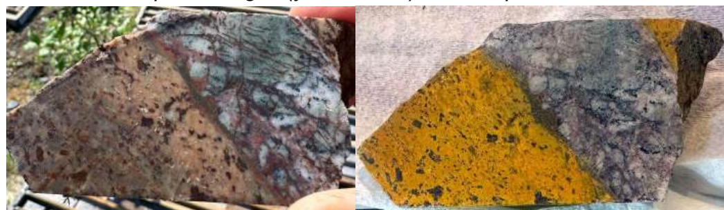
Intense K-feldspar selvages (yellow stain) around qtz-sulfide vein 189.5m
