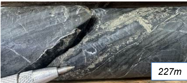
Mudstones with sulfide laminae 3.5 ppm Ag 859 ppm Cu / 2m (228-228m)
