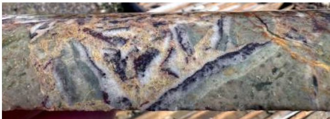
Intense K-feldspar selvages (yellow stain) around qtz-sulfide vein 189.5m
