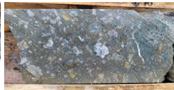
TC20-02 (69.8m) Polymictic breccia (0.85% Cu, 0.11 g/t Au, 20.2 g/t Ag / 1.12m (69-70.12m))
