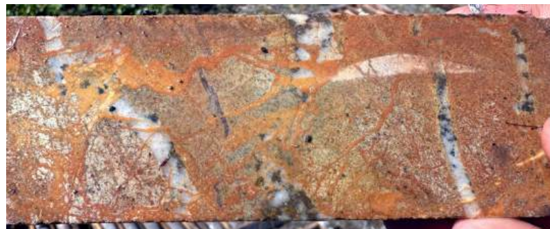
Quartz-sulfide veins cut by carbonate stockwork 0.303 g/t Au 0.19% Cu; 253.1m
