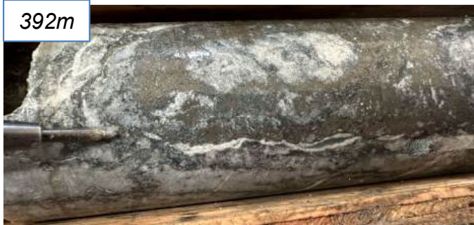
Black chlorite-sulfide veins 358 ppm As 18 ppm Sb / 3m (391-394m)
