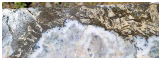
TC20-02 (18.6m) quartz-carbonate-sulfide epithermal vein (0.798% Cu, 23.6 g/t Ag, 0.96% Zn / 0.5m , 18.43-18.93m)
