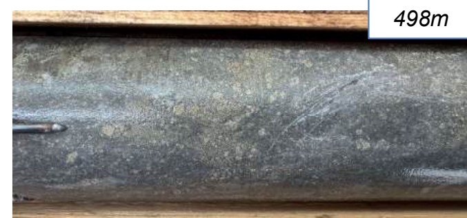
Pyrite flooded feldspar phyrlic andesite: 0.15 g/t Au 2.5 ppm Bi 14.1 ppm Te 23 ppm Se / 3m (495-498m)
