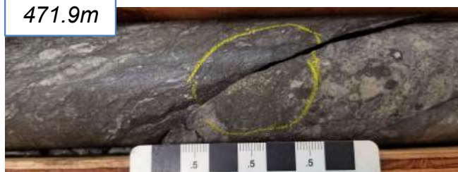
Intensely sericite altered andesite, breccias with sulfide clasts / matrix, anomalous Cu-As(±Au) 122 ppm Cu 314 ppm As / 1.68mm (471.45-473.13m)
