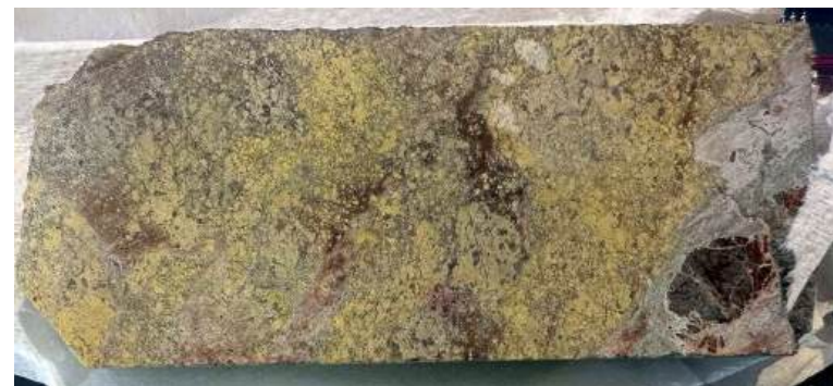
Quartz-sulfide veins cut by carbonate stockwork 0.303 g/t Au 0.19% Cu; 253.1m
