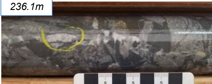
Brecciated andesite flow with mud matrix 190 ppm As / 3m (236-239m)
