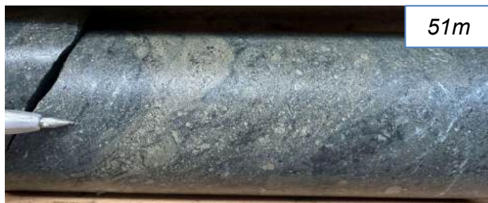
Sulfide flooded domain in chlorite altered andesite fragmental: 0.085 g/t Au 410 ppm Cu / 3m (48-51m)
