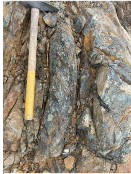
A0420662: brecciated mudstone+sulfides 2.87% Cu
