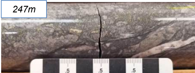
Quartz-carbonate-pyrite-chalcopyrite breccia 378 ppm Cu 267 ppm As / 3m (245-248m)
