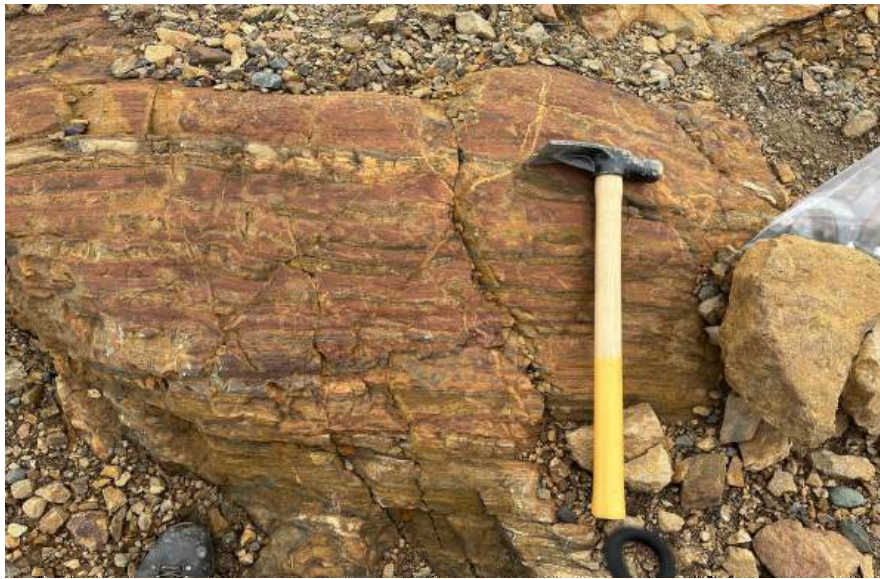
Well bedded siliceous mudstones with pyrite laminae
