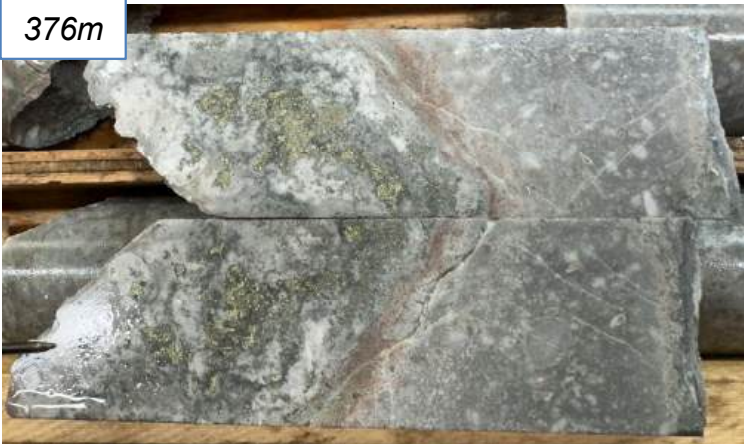
Quartz-chalcopyrite vein in porphyry 86 ppb Au 674 ppm Cu / 3m (373-376m)
