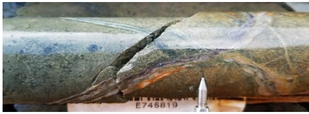
Drill hole photos of NQ core, diameter 47.6 mm
