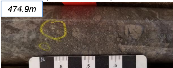
588 ppm Cu 296 ppm As / 3.59m (473.13-476.72m)
