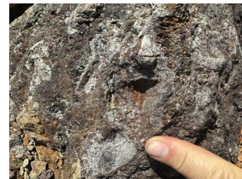
L615119: hydrothermal breccia with chalcopyrite-pyrite rich matrix 262 g/t Au, 2.46% Cu
