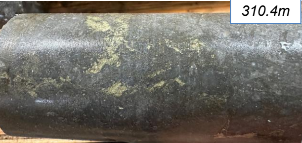
Chalcopyrite veins in andesite breccia 930 ppm Cu / 3m (308-311m)
