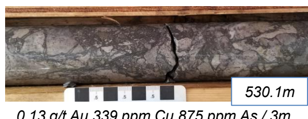
0.13 g/t Au 339 ppm Cu 875 ppm As / 3m (528-531m)
