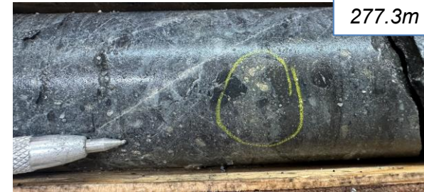
Hydrothermal breccia 444 ppm Cu 14 ppm Mo / 3m (276-279m)
