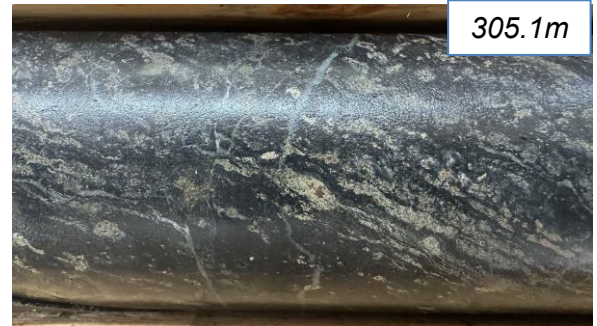
Mudstone with sulfide laminae 538 ppm Cu 36 ppm Mo 17 ppm Sb / 3m (303-306m)
