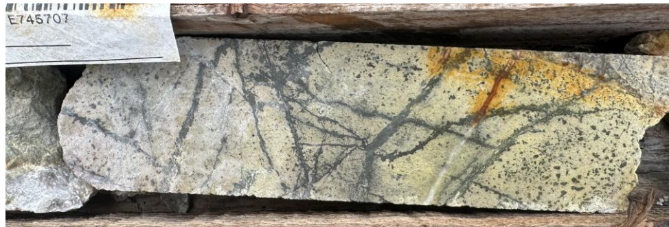
Sulfide stockwork, QSP alteration 0.14% Cu, 0.23% Zn
