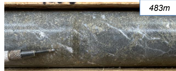
Sericite-pyrite-calcite altered volcanics: 75 ppb Au 13.2 ppm Te / 3m (480-483m)
