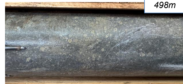
Pyrite flooded feldspar phyrlic andesite: 0.15 g/t Au 2.5 ppm Bi 14.1 ppm Te 23 ppm Se / 3m (495-498m)
