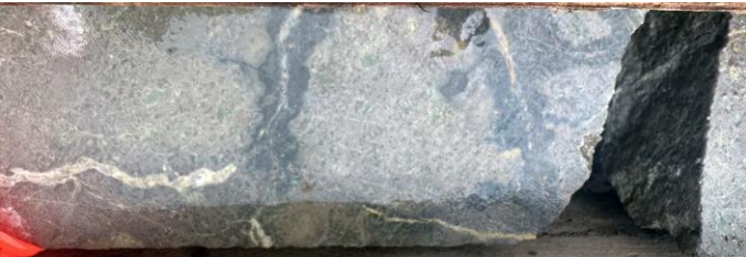
TC20-01 (156m) py-aspery and quartz veins in tuff with disseminated py and purple anhydrite
