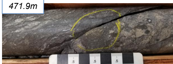
122 ppm Cu 314 ppm As / 1.68mm (471.45-473.13m)
