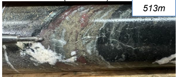
655 ppm Cu 26 ppm Mo 25 ppm Sb / 2m (512-514m)
