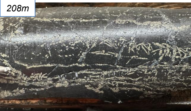
Hematitic mudstone with pyrite 189 ppm Cu 15 ppm Mo 173 ppm As / 3m (207-210m)
