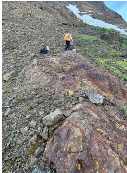
L615116: QSP altered conglomerate cut by NNW trending shear 5.8 g/t Au, 3.31% Cu
