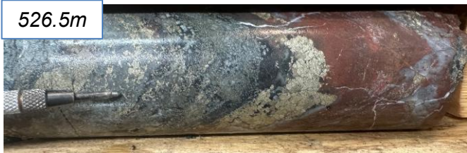
419 ppm Cu 37 ppm Mo 15 ppm Sb / 2m (526-528m)
