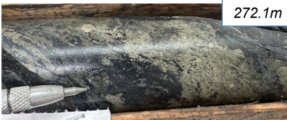
Semi-massive sulfides in mudstone 83 ppb Au 786 ppm Cu 38 ppm Mo 164 ppm As / 3m (270-273m)
