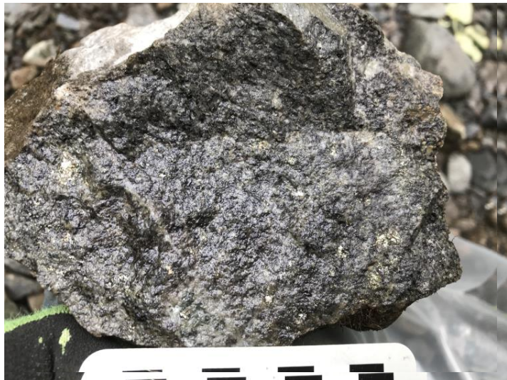
S850066 Creek float of fine grained biotite altered intrusive with disseminated cp and Qtz-cp-py veinlets; 0.30% Cu, 0.1 g/t Au
