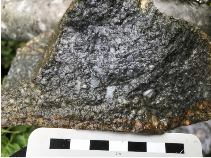
S850067 Creek float of quartz-feldspar-biotite porphyry with sericite-pyrite altered groundmass; 320 ppm Cu
